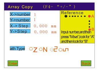
Method I: Input the quantity of array copy in X direction and Y direction; then press "MOVE" key and move to the last point of X direction (point A in the figure) and press "confirm"; then move to the last point of Y direction (point B in the figure) and press "confirm"; automatically calculate the distance. First input the copy quantity. Route method: selection of operation trace.
