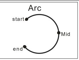
Press figure key 3 and enter into the arc command edition screen; first edit the starting point coordinate of arc, then middle point coordinate and ultimately terminal coordinate. The edition methods are same as the "point" edition methods.
