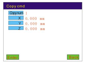
Method I: Input copy quantity; if distance between copied command coordinates is clearly known, directly input coordinate distance of "X""Y""Z" (distance between coordinates); press "confirm" key and complete the copy.
