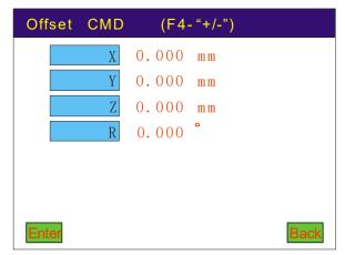
Method I: Input specific offset data and press "confirm" key and complete the offset.
